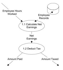
You should notice that the flows in and out of this diagram are exactly the same as those into and out of the previous bubble, but that there is now an extra flow within. Of course, this extra flow needs documentation.
