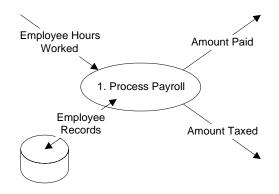
The initial step would be to draw out the single bubble for the system, and to draw the inputs and outputs in. Note that the arrows are data items, and are named using nouns, while the bubble itself is a process, and therefore is named using a verb. This naming method will be used throughout. This is the top level **Data Flow Diagram**, or DFD for short.
